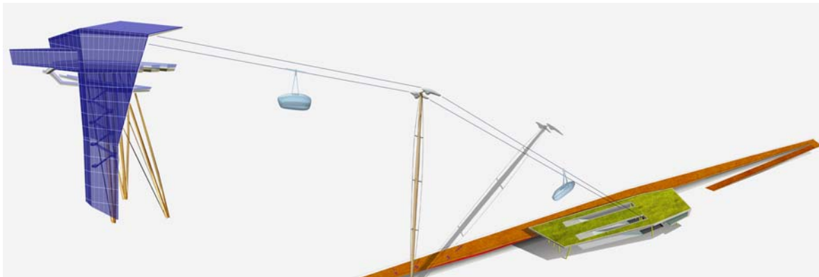
A composite image showing the upper terminus on the left, the mast-like supporting tower in the center and the "subterranean" lower terminus on the right.
